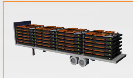
Transportable by standard freight, 6 stacked shutters, 24 shutters per truck trailer (2.8m x 2.5m).
